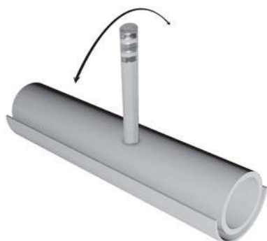
Fig. 8.4 Directions of movement allowed by a hinge like joint
