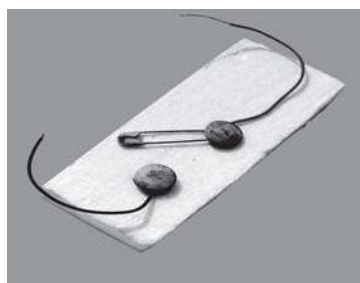
Fig. 12.8 A simple switch
