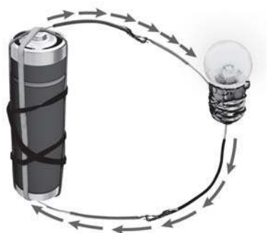
Fig.12.6 Direction of current in an electric circuit
