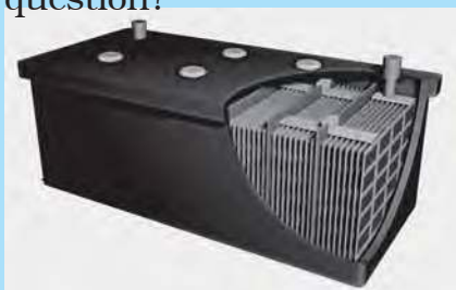
Fig. 14.6 Truck battery and its cutout
