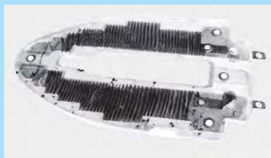
Fig. 14.11 Element of electric iron
